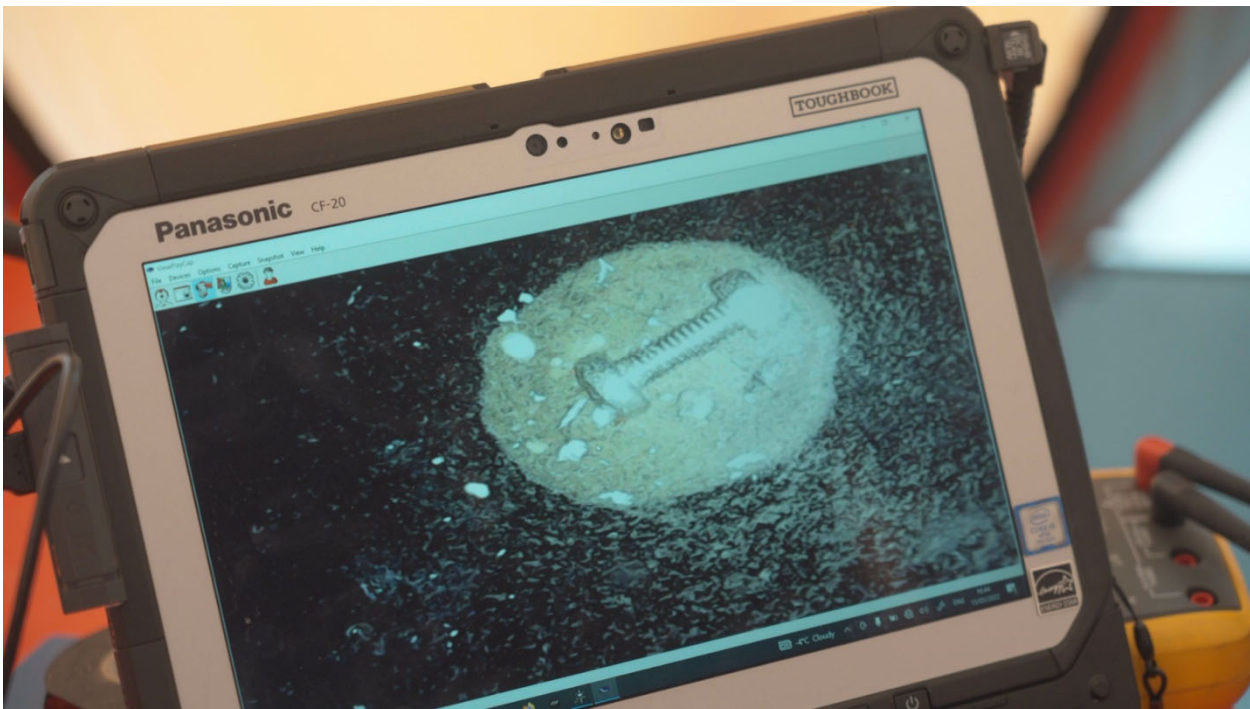
795 | Figure 219 – Down-borehole video camera shows substantial sediment accumulation on the borehole bottom within 5 m of the ice surface. We estimate that a water-filled cavern of diameter ~50 cm formed around the melt tip. A bolt of length ~1.5 cm was dropped into the frame for scale.
