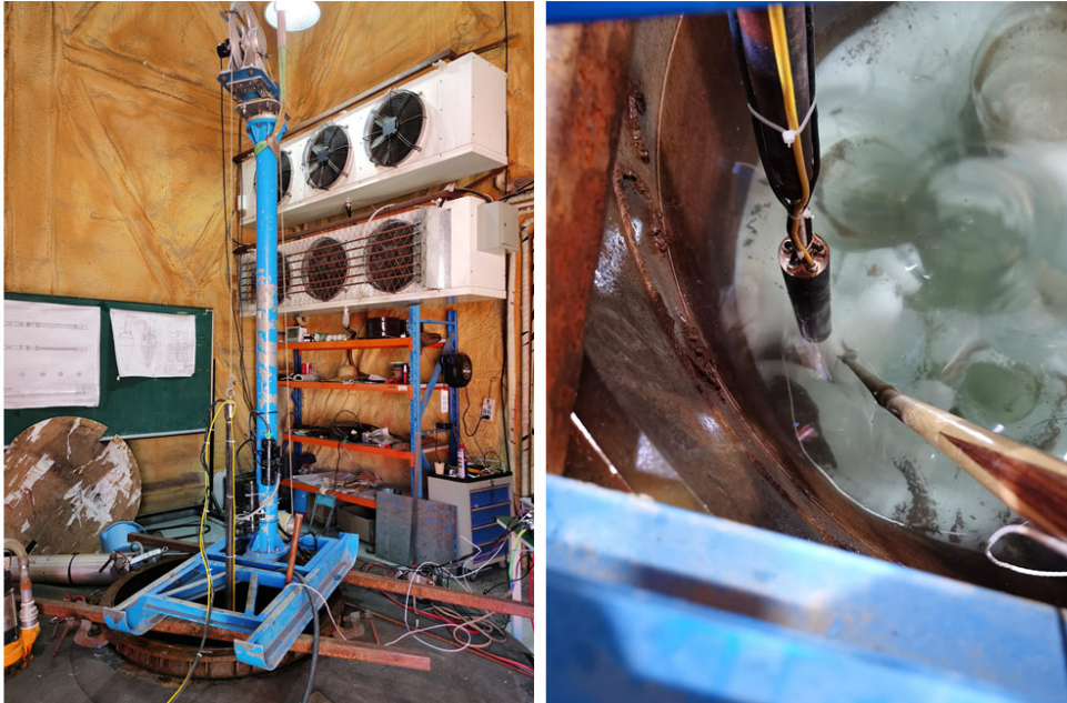
Figure 14 – Left: The melt tip is attached to a 2 m drill flight and suspended from an oversized winch above the ice well during laboratory testing. Right: Looking down into the ice well as the melt tip starts a new borehole. A matrix of previous boreholes is seen in the ice well.
