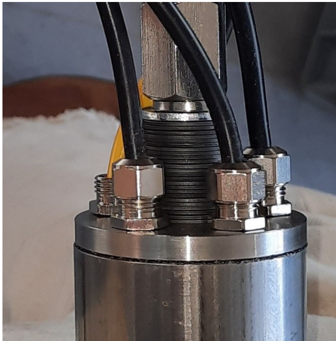
Figure 6 – With four power cables, one data cable and an M10 threaded bolt covered in Belleville washers, there is very little free space on the metal top cap of the lower member of the melt tip.
