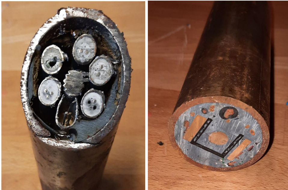
830 Figure 17-18 – Melt-tip cross sections from destructive testing of the v2 melt tip. Left: The resin filling encasing the unheated portions of the cartridge heaters resin exposed from the copper heating block has melted. Right: Uncompromised resin filling higher in the melt tip, encasing the electronics package.
