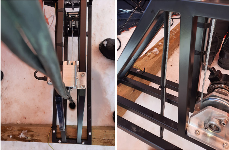
Figure 87 – Overhead (Left) and side (Right) views of the umbilical cable bundled with zip ties prior to entering the borehole.
