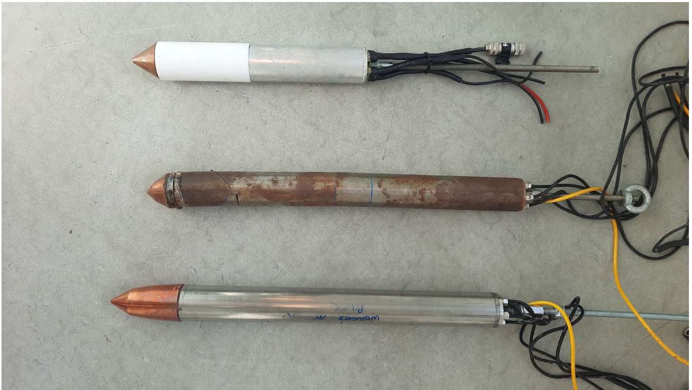
760 | Figure 32 – Photograph of the v1 (top), v2 (middle) and v3 (bottom) melt tip versions developed over the three-year project lifetime (v0 not shown). The v2 melt tip shown here, which has been sectioned for destructive testing, bears a characteristic rust coating that develops with melt tip use. The v1 and v3 melt tips shown here have not been used.
