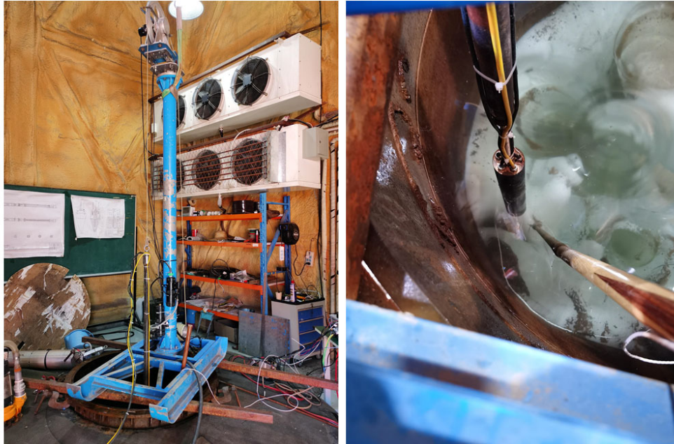
815 Figure 14-15 – Left: The melt tip is attached to a 2 m drill flight and suspended from an oversized winch above the ice well during laboratory testing. Right: Looking down into the ice well as the melt tip starts a new borehole. A matrix of previous boreholes is seen in the ice well.
