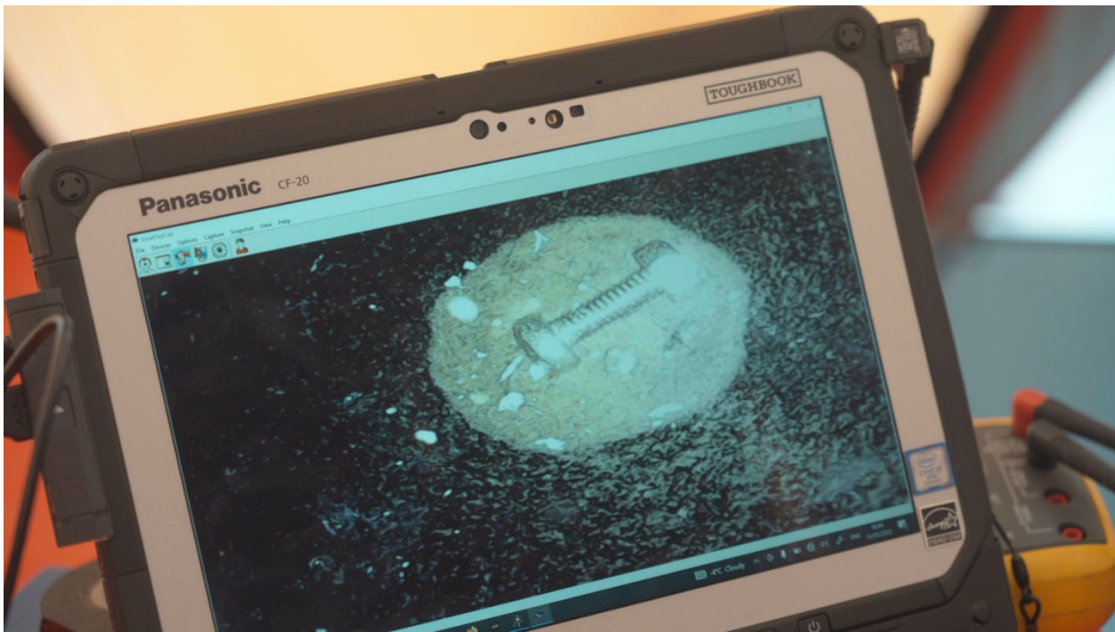
850 | Figure 21-22 – Down-borehole video camera shows substantial sediment accumulation on the borehole bottom within 5 m of the ice surface. We estimate that a water-filled cavern of diameter ~50 cm formed around the melt tip. A bolt of length ~1.5 cm was dropped into the frame for scale.
