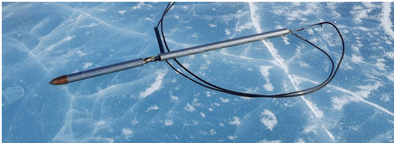
Figure 5 – Photo of a fully assembled v3 melt-tip on lake ice. The lower member (image left) is sealed and resin-filled while the upper member (image right) is unsealed and unfilled.
