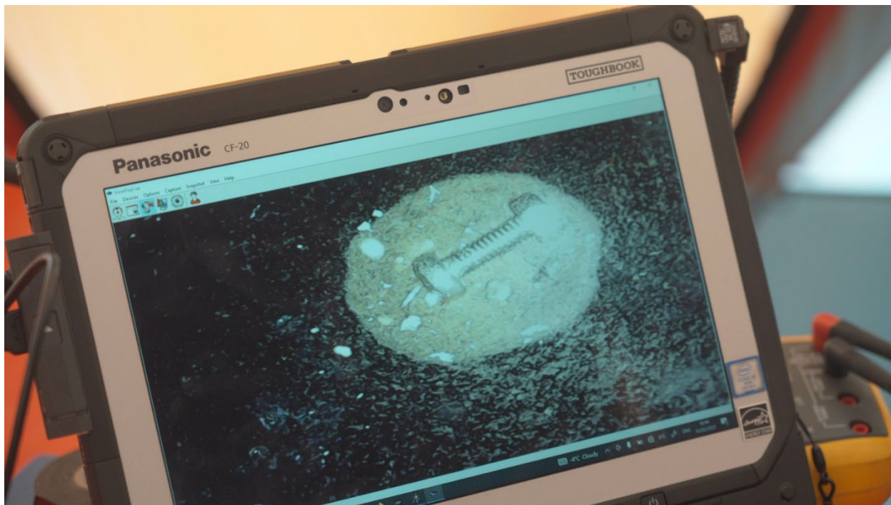
Figure 21 – Down-borehole video camera shows substantial sediment accumulation on the borehole bottom within 5 m of the ice surface. We estimate that a water-filled cavern of diameter ~50 cm formed around the melt tip. A bolt of length ~1.5 cm was dropped into the frame for scale.
