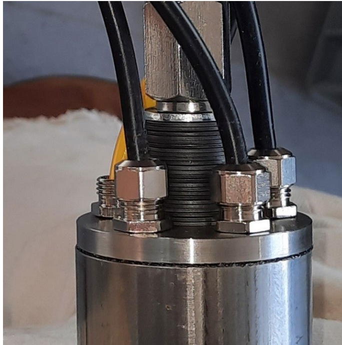
770 Figure 7 – With four power cables, one data cable and an M10 threaded bolt covered in Belleville washers, there is very little free space on the metal top cap of the lower member of the melt tip.
