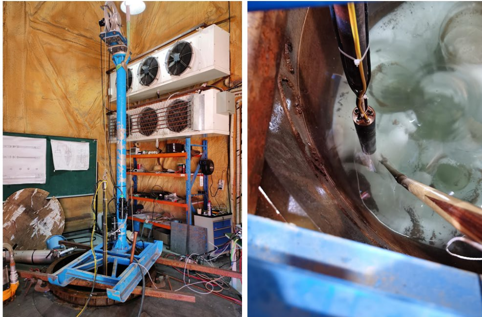
Figure 15 – Left: The melt tip is attached to a 2 m drill flight and suspended from an oversized winch above the ice well during laboratory testing. Right: Looking down into the ice well as the melt tip starts a new borehole. A matrix of previous boreholes is seen in the ice well.
