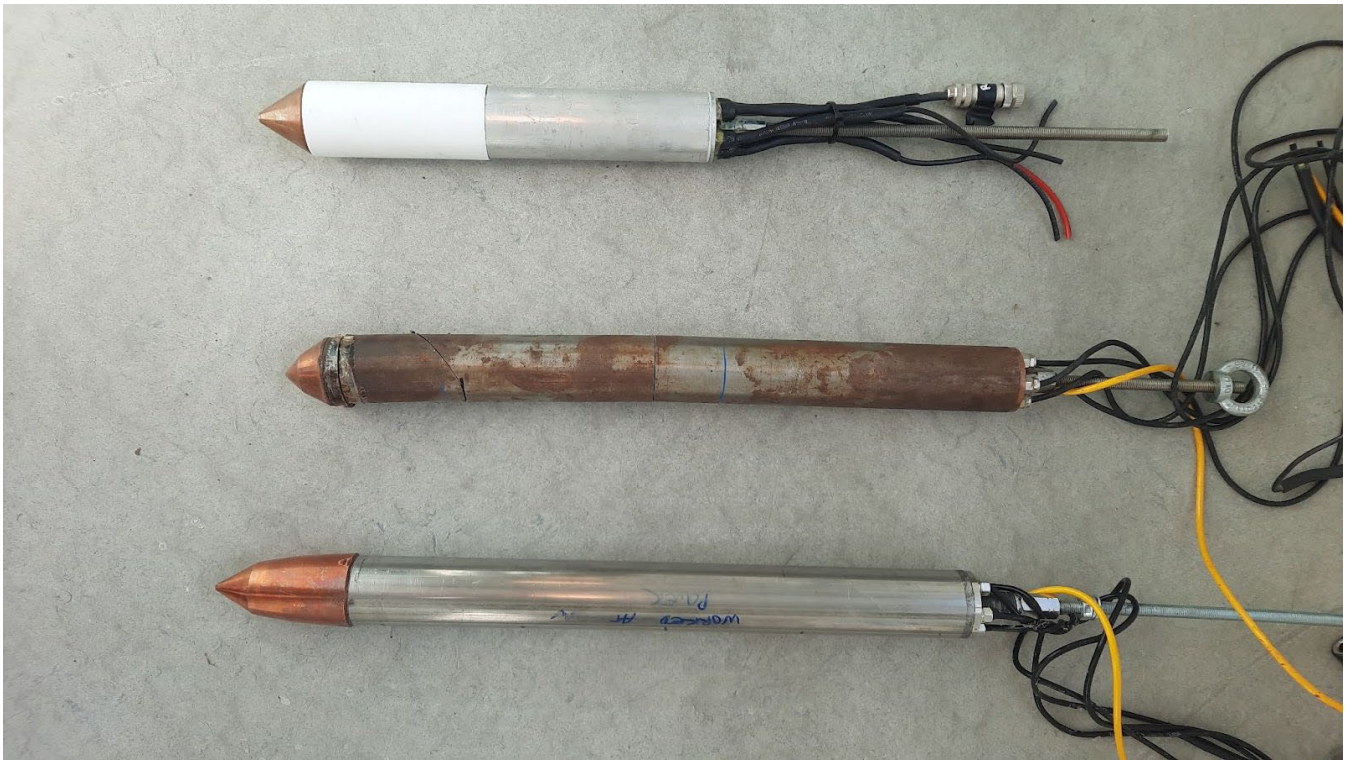
Figure 3 – Photograph of the v1 (top), v2 (middle) and v3 (bottom) melt tip versions developed over the three-year project lifetime (v0 not shown). The v2 melt tip shown here, which has been sectioned for destructive testing, bears a characteristic rust coating that develops with melt tip use. The v1 and v3 melt tips shown here have not been used.
