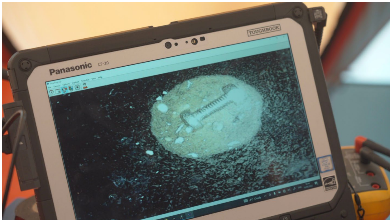
Figure 22 – Down-borehole video camera shows substantial sediment accumulation on the borehole bottom within 5 m of the ice surface. We estimate that a water-filled cavern of diameter ~50 cm formed around the melt tip. A bolt of length ~1.5 cm was dropped into the frame for scale.
