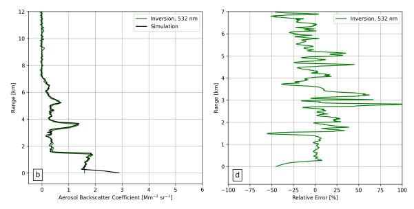
**Figure 5** - Left panels show a comparison of the aerosol backscatter coefficient (Mm-1 sr-1) retrieved at (a) 355 nm (blue) and (b) 532 nm (green) with those used as input for the simulation (black line). The right panels show the respective relative errors (%).
