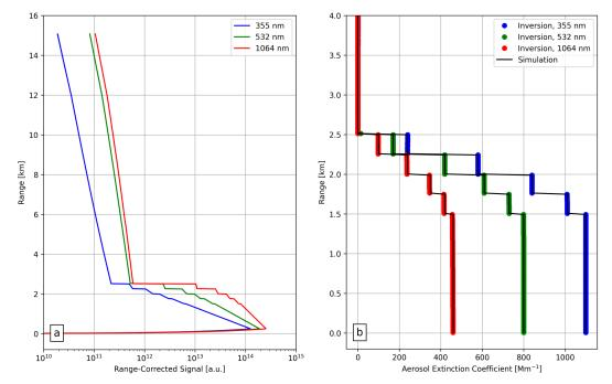
*Figure 3 -* (*a*) Synthetic Range-corrected signals (*a.u.*) and (*b*) aerosol extinction coefficients (*Mm*<sup>-1</sup>) retrieved with LPP (bullets) and used as input for the simulation (black line) are shown for 355, 532 and 1064 nm.
