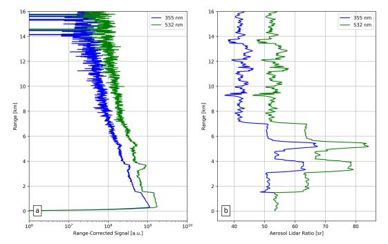
*Figure 4 -* (a) Synthetic Range-corrected signals (a.u.) with raw vertical resolution of 15 m and (b) aerosol lidar ratio (sr) used as input for the simulation are shown for 355 nm and 532 nm. The retrievals shown in Fig. 6 assumed constant lidar ratios of 51 sr and 62 sr, respectively.
