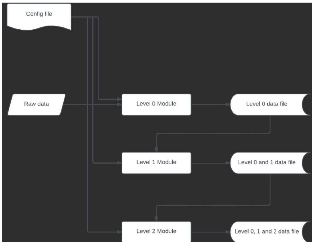
Figure 1. Flow diagram showing the structure of LPP version 1.1.0. Each module receives as input the data file produced as output in the previous module. A single configuration file is used for all the modules.
