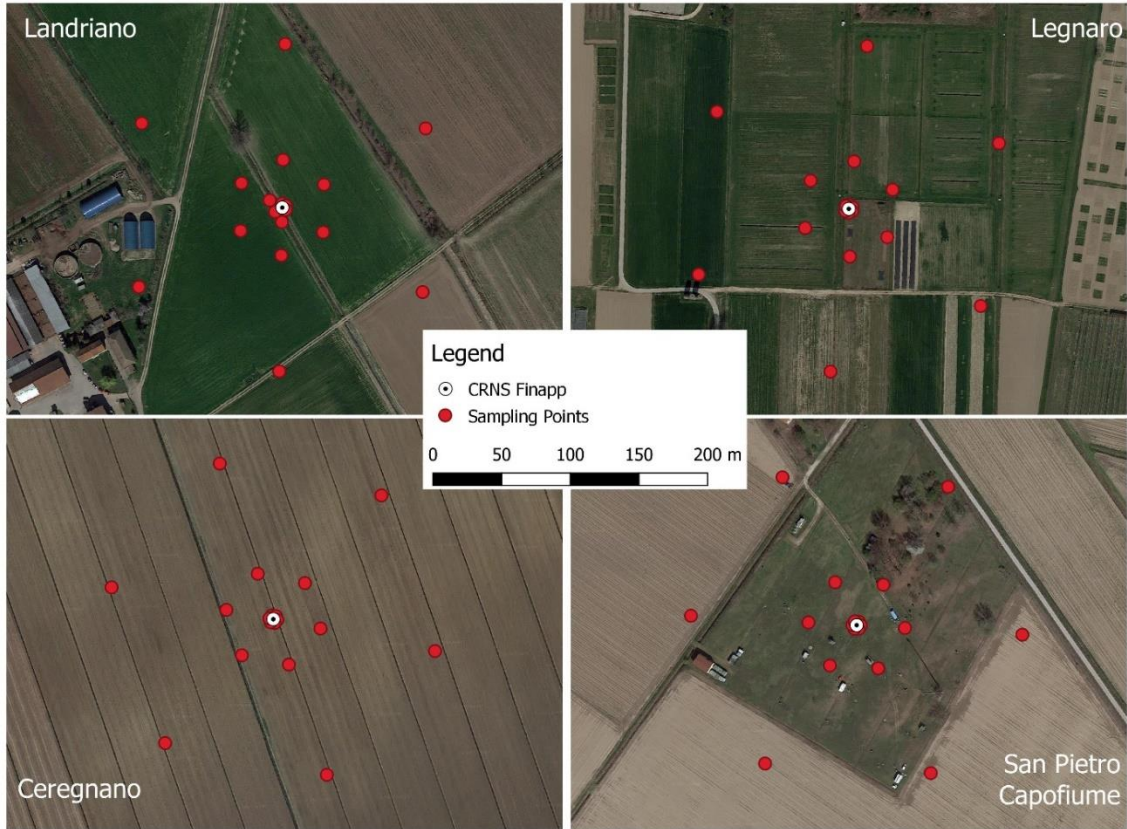
Figure 3. Experimental sites with FINAPP3 sensor (white points) and locations where gravimetric soil samples (red points) have been collected for comparison (pictures from Google Earth).
