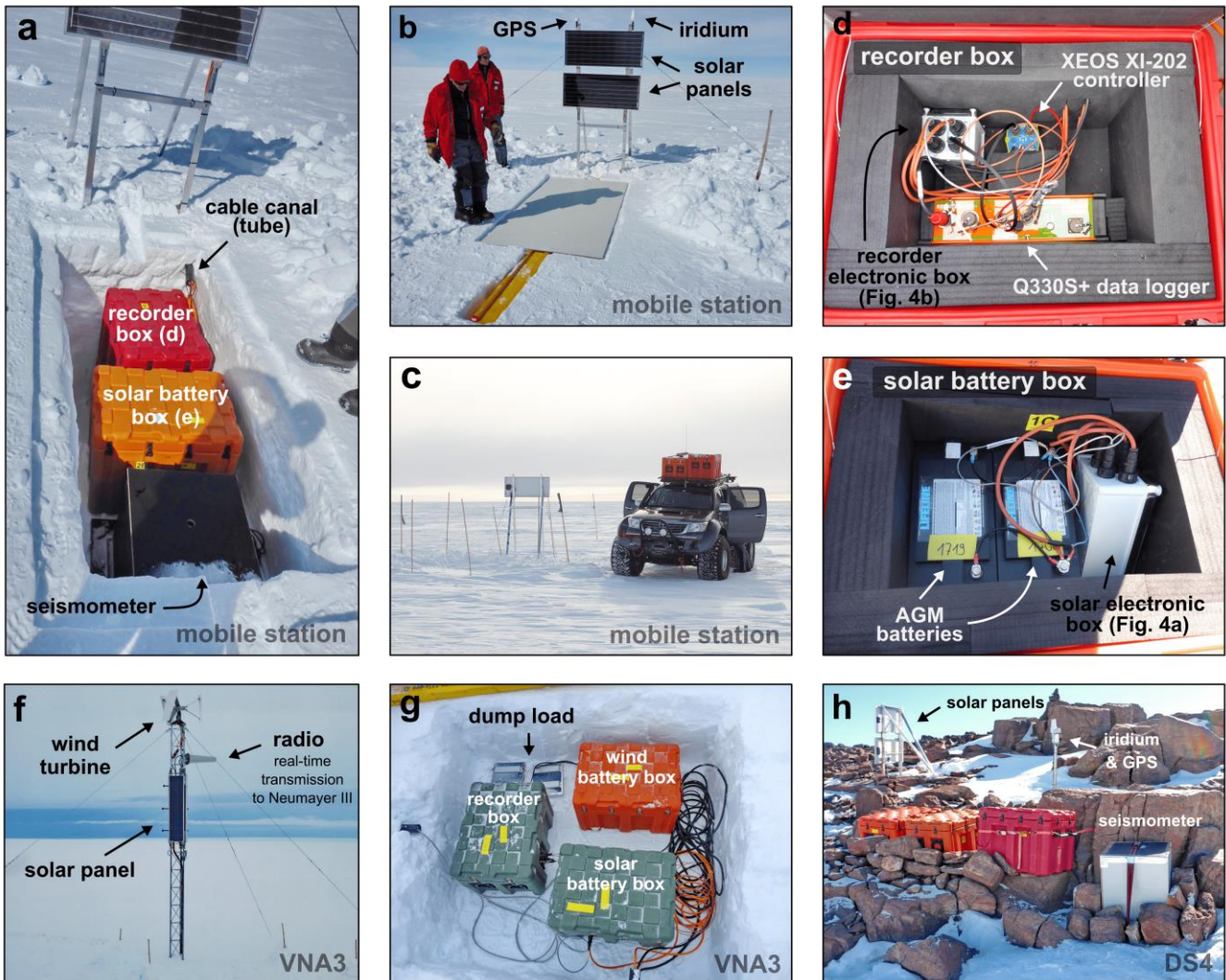
Figure 3: Photographs of the station design from several deployments in western Dronning Maud Land (East Antarctica). Panels (a–c) show the setup of the mobile stations on the ice surface. Panels (d) and (e) show the recorder and solar battery boxes from the inside. The permanent real-time station setup of VNA3 is shown in (f) for the ice surface and in (g) for the ice cave. Panel (h) shows the station layout of DS4, which is deployed on a rock base. Photo credits: (a,b, d-h) Jölund Asseng; (c) Steven Franke.
