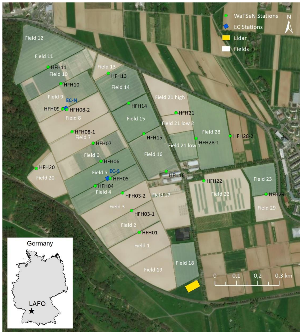
Figure 2 LAFO experimental site at the Heidfeldhof, locations of the two eddy covariance stations, the 22 soil water content and temperature stations, remote sensing equipment at the lidar site, and extents of agricultural fields. The inlet shows the location of LAFO in Southwest Germany. Basemap source: Esri, DigitalGlobe, GeoEye, Earthstar Geographics, CNES/Airbus DS, USDA, USGS, AeroGRID, IGN, and the GIS User Community.
