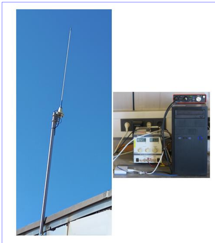
Figure 2. Photo of the new reception system in operation since 2019. The left and right panels display, respectively, the new antenna (i.e., Procom BCL 1-KA) rigidly fixed on a pole and installed on the roof of the building/institute, and the detected radio signal is processed/digitized by a sound card Focusrite Scarlett 2i2 which is connected to a PC running under a Linux operating system. The electronics boxes, power supply, and connecting cables are in an air-conditioned environment. The compact arrangement of devices still enables easy maintainability.
