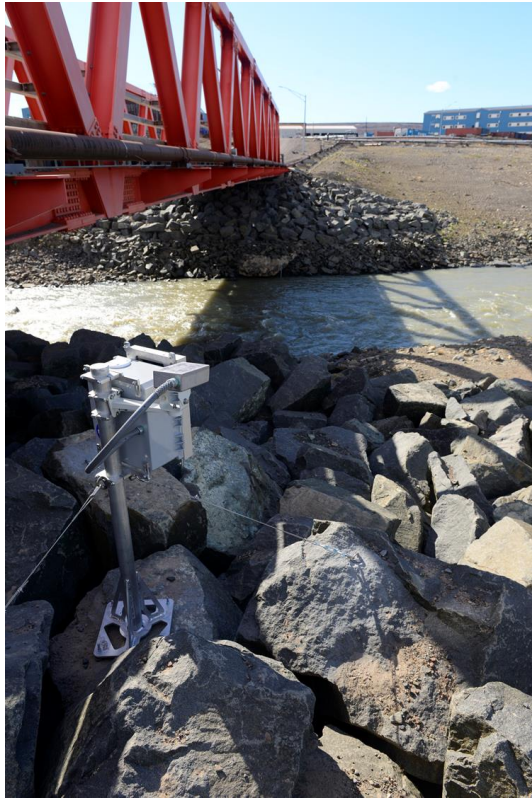
Figure 3: Bank-mounted, oblique-looking Laser rangefinder recording river stage on the right bank of the North River, Thule AB. In total, four identical Laser rangefinder units were built and installed in NW Greenland, with two at the Minturn River (Inglefield Land), one at the North River (Thule AB), and one at Fox Canyon River (Thule AB). The single-shot Laser rangefinder measures distance between the sensor and water surface using time-of-flight of the emitted and reflected beam. This novel approach to river stage measurement avoids contact with water, reducing risk of sensor damage or loss from ice, rolling cobbles, and spring breakup floods (photo by Lincoln Pitcher).
