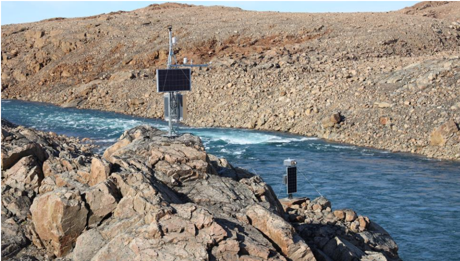
525 Figure 4: Automated weather station and CF Bubbler vented pressure transducer (at left) and a time-lapse camera (at right) established at the Minturn River. Other instruments at this site include two bank-mounted laser rangefinders, a second vented P pressure transducer, and a second time-lapse camera on the opposite bank (photo by Lincoln Pitcher).
