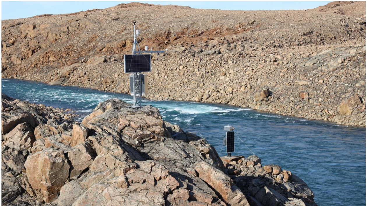
485 Figure 4: Automated weather station and CF Bubbler vented pressure transducer (at left) and a time-lapse camera (at right) established at the Minturn River. Other instruments at this site include two bank-mounted laser rangefinders, a second vented pressure transducer, and a second time-lapse camera on the opposite bank (photo by Lincoln Pitcher).
