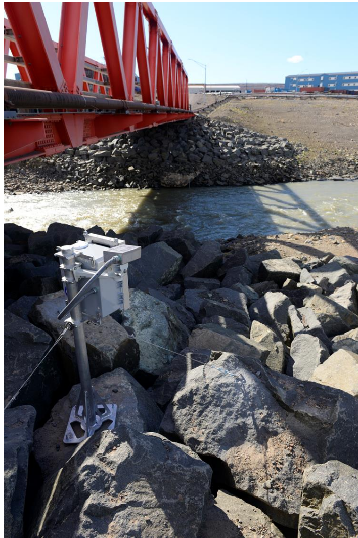
475 Figure 3: Bank-mounted, oblique-looking Laser rangefinder recording river stage on the right bank of the North River, Thule AB. In total, four identical Laser rangefinder units were built and installed in NW Greenland, with two at the Minturn River (Inglefield Land), one at the North River (Thule AB), and one at Fox Canyon River (Thule AB). The single-shot Laser rangefinder measures distance between the sensor and water surface using time-of-flight of the emitted and reflected beam. This novel approach to river stage measurement avoids contact with water, reducing risk of sensor damage or loss from ice, rolling cobbles, and spring breakup 480 floods (photo by Lincoln Pitcher).
