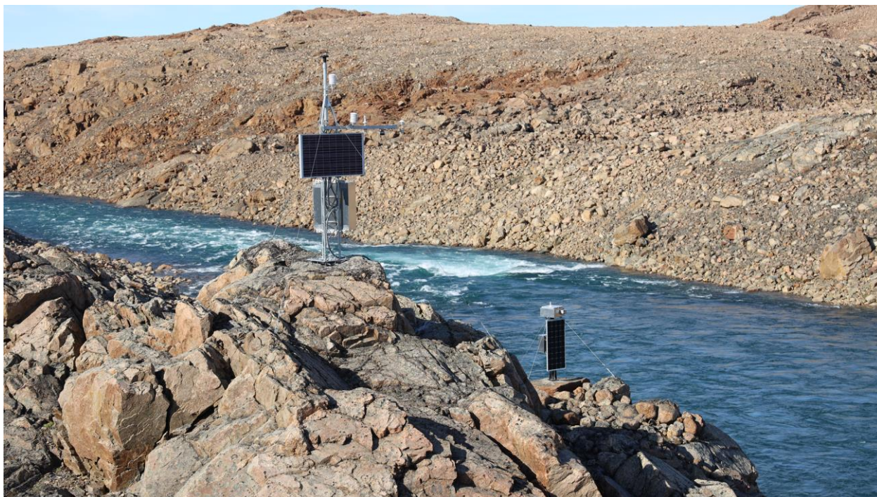
485 Figure 4: Automated weather station and CF Bubbler vented pressure transducer (at left) and a time-lapse camera (at right) established at the Minturn River. Other instruments at this site include two bank-mounted laser rangefinders, a second vented pressure transducer, and a second time-lapse camera on the opposite bank (photo by Lincoln Pitcher).
