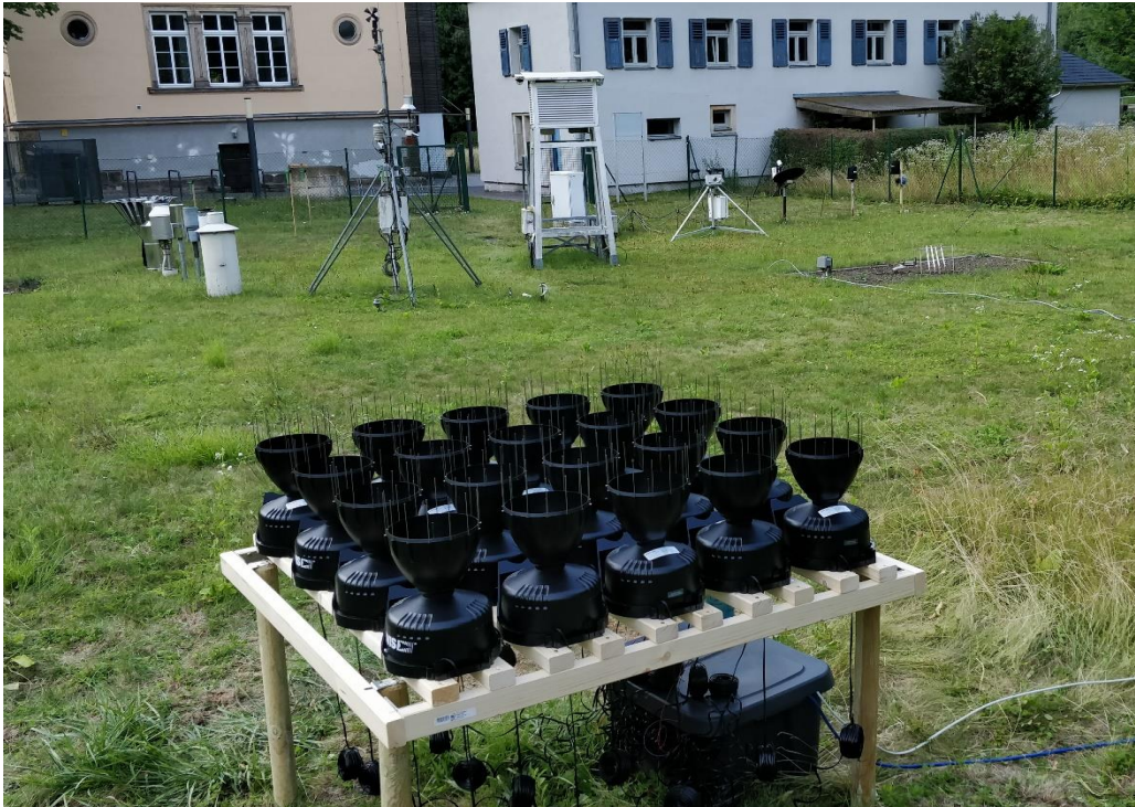
Figure 2: Tharandt meteorological site with reference instruments (in background on the left side) and field study setup (in foreground)
