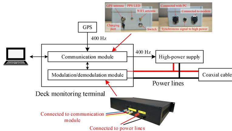
109 **Fig.3** The block diagram of deck monitoring terminal.
