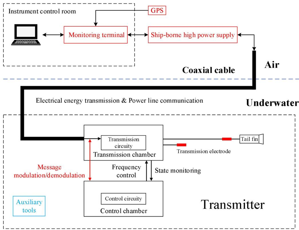
Fig.1 The schematic diagram of MCSEM transmission system based on coaxial cable.
