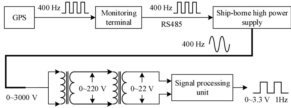
Fig.2 The flow diagram of synchronization signal.
