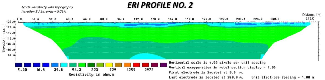
**Figure 7: ERI profile No. 2 at the Rospuda site - inverted resistivity model with topography.**
