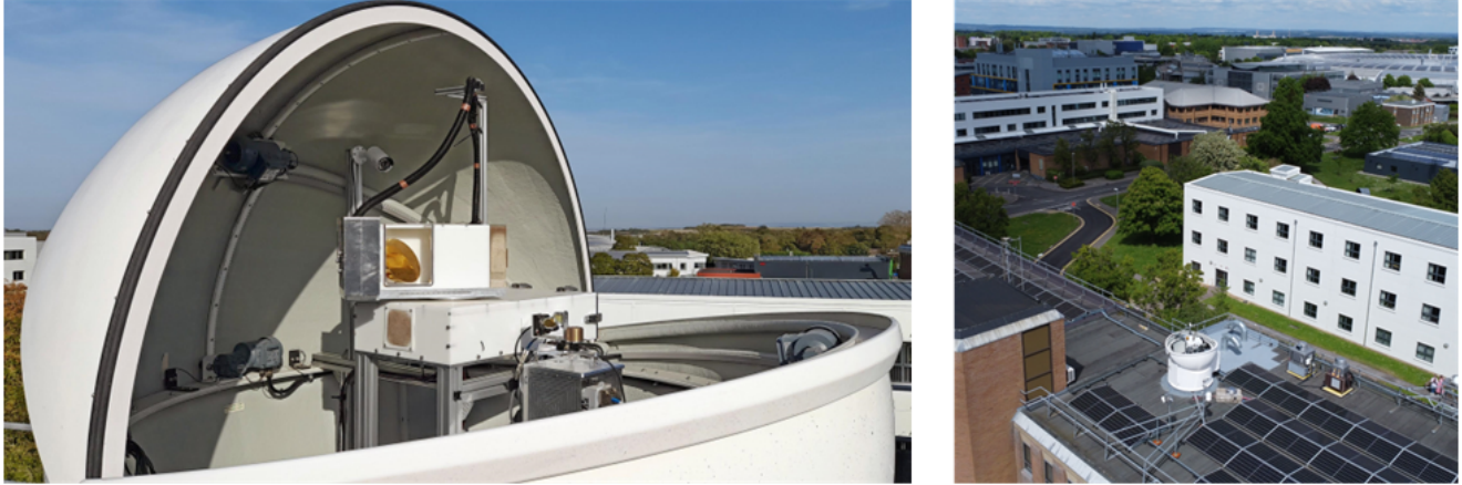
Figure 3. Left, view of the alt-azimuth high pointing precision solar tracker operating in the astronomical dome. Right, general view of the roof installation within the Harwell Campus (Drone image courtesy of Melina Zempila).
