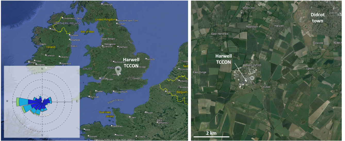
Figure 1. Harwell TCCON setting. Left, general site location within the UK. The insert in the bottom left gives the diurnal wind rose from the site wind measurements for September 2022 to September 2023. Dark blue, light blue, and green correspond to 1-3, 3-5, and 5-7 m/s bins, respectively. The coordinate circles are spaced every 5% frequency intervals. Right, Close-up of the Harwell scientific campus indicating the mostly rural surroundings, apart for the small town of Didcot in the north-east. Background images ©Google Earth.
